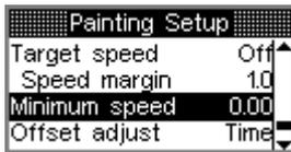
When minimum speed threshold is set to zero, the output testing page will have to be accessed from the operating menu.
