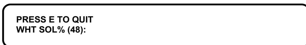
**Step 5** Use the LHK number keys to enter the paint solids volume for the white paint and press **ENTER**
