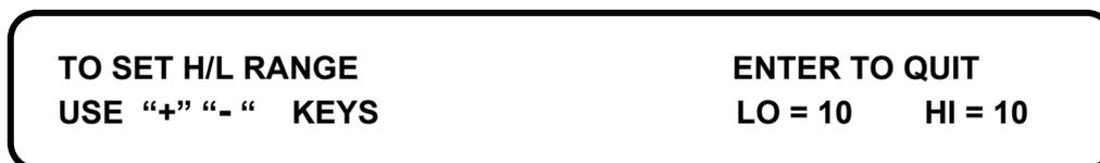
**Step 3** Use the **+** and **-** keys on the LHK to change the LO speed setting and use the **+** and **-** keys on the RHK to change the HI speed setting.
