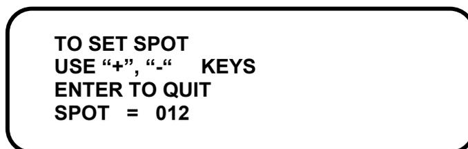
**Step 3** Use the +, - Keys to adjust the line spot length. **Note:** This amended spot length will now apply to all spot patterns.
